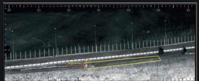
Zones with smart alarm conditions for human intrusion detection and tracking
