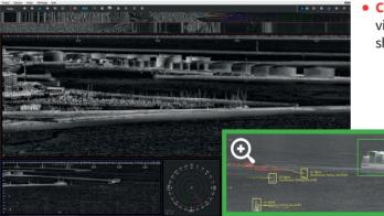
CYCLOPE Software user interface displaying real-time panoramic videos with automatic classification (performed here per class of ship).
