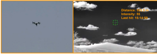
Visible and IR views with threat distance provided by the Laser Range Finder
