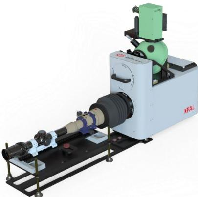
HGH, world leader in Electro-optics test equipment, based in Igny near Paris, entirely renewed their range of **field collimators** to support this project. The **OPAL collimator** is a compact and versatile portable collimator enabling the maintenance in the field of many other electro optics systems such as goggles, visible to IR cameras and laser rangefinders.
