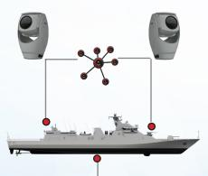
**2. Data** is processed by **CYCLOPE Hypervisor** software collecting, displaying and fusing on a **single workstation**, all the threats automatically detected and tracked by the two SPYNEL sensors.
