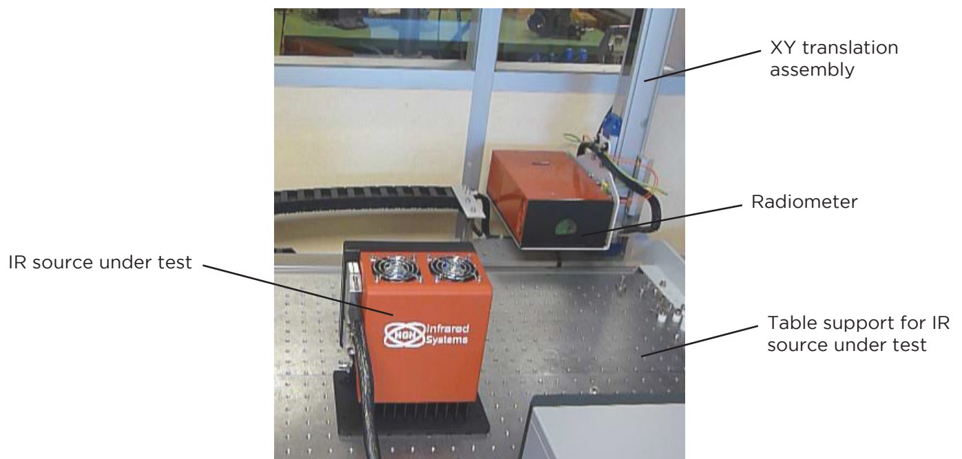
Figure 5 Overview of the IR sources uniformity measurement bench
