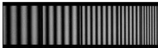
Figure 1 : Sinewave target of various spatial frequencies .
