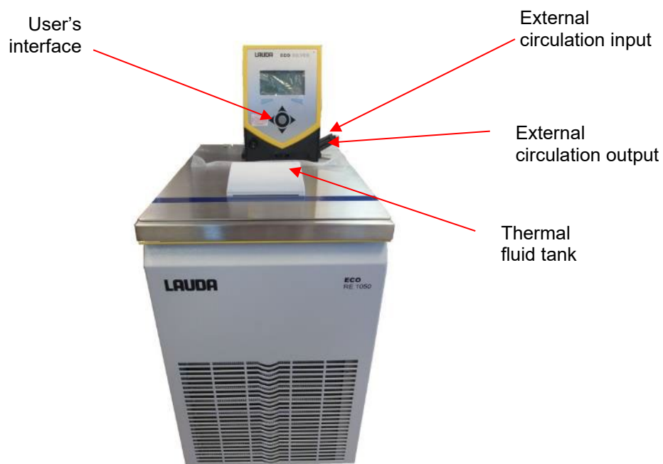
Figure 11: Lauda Thermostat front view
