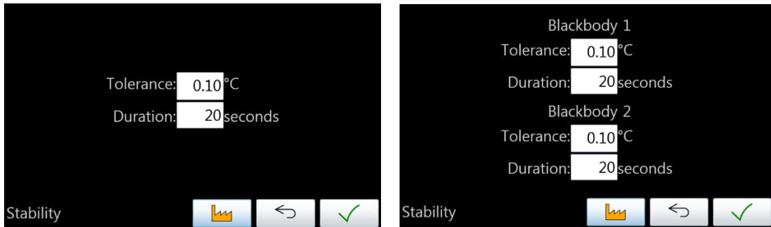
Figure 17 : Stabilization menu screen, left: 1 head connected / right : 2 heads connected
