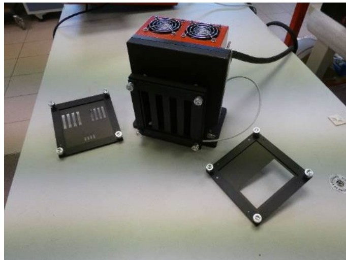
Figure 21: DCN 1000 H4 mounted with target holder and targets
