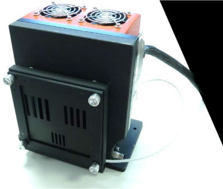
Figure 17 : DCN 1000 H4 blackbody with mounted MRTD target
