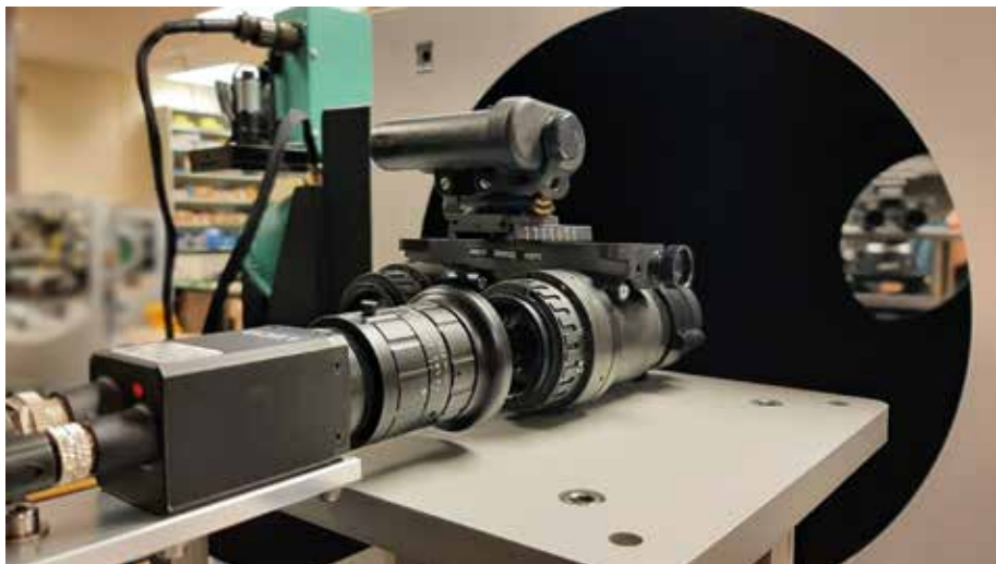
HGH's eye-camera collecting a high resolution image through the eyepiece
