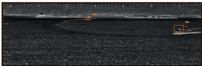
Small boat detection, tracking and classification with Cyclope software
