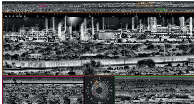
Cyclope GUI for onshore facility monitoring
